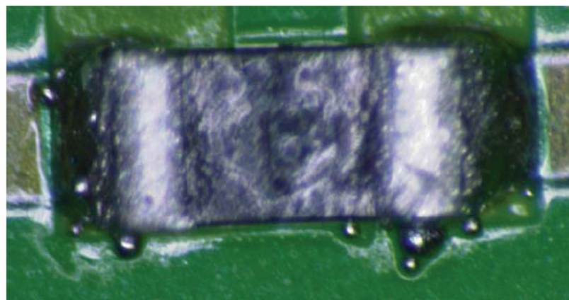
b) 400 thermal Cycles (-55/100°C)
