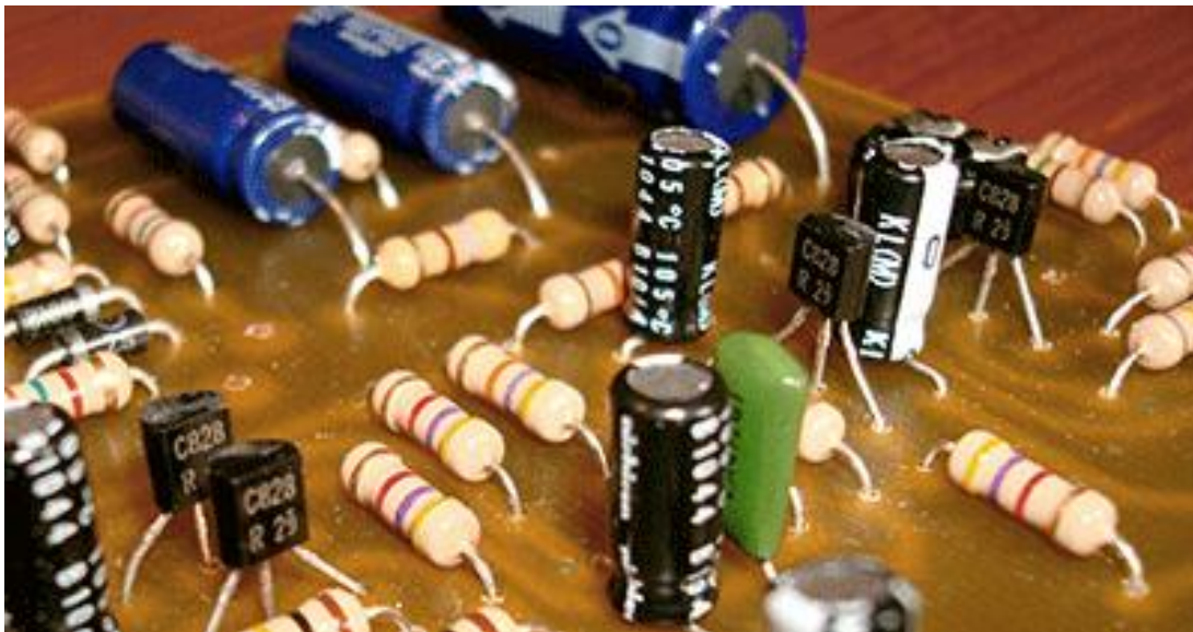
Figure 1: Carbon Resistors (as noted by their color rings)
