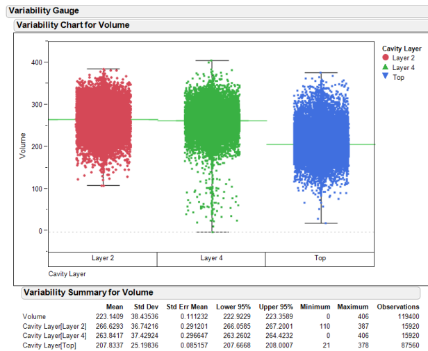
Figure 12. Solder paste volume by board cavity location.
