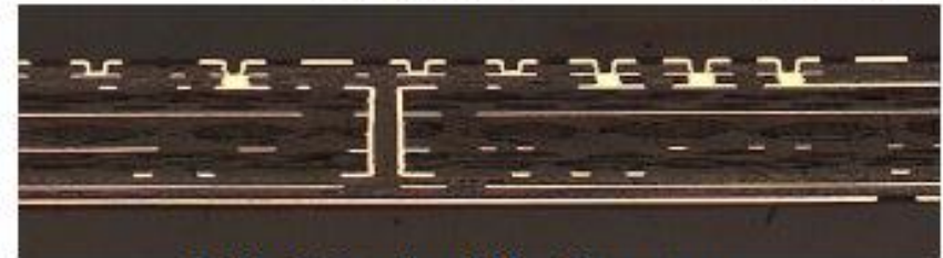
2+N+2 Stacked Via Structure
