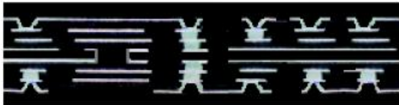
3+N+3 Stacked Via Structure
