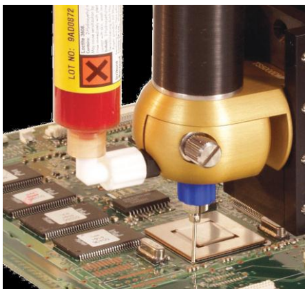
Figure 12: Dispensing epoxy underfill
