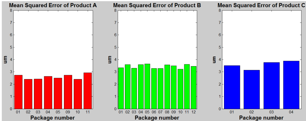
Fig. 8. MSE of calculated ball height results compared to confocal results for three products.
