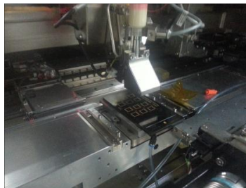
Figure 6: Flip chip bonding process.
