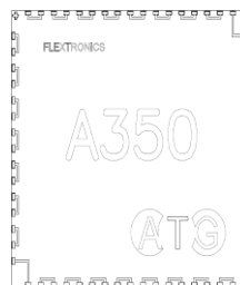
Test die daisy chained pads
