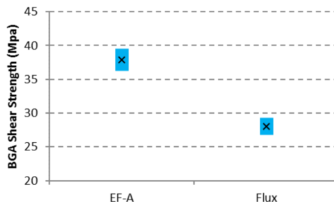
Figure 13 Shear strength of a BGA assembled with epoxy flux A and a conventional flux
