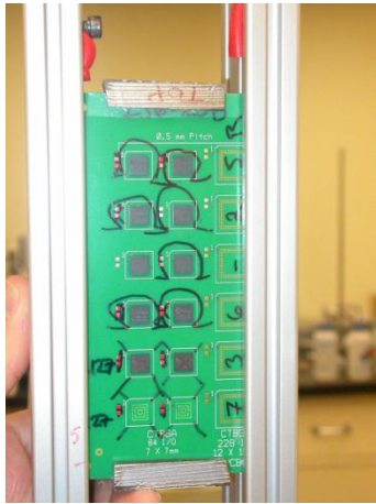
Figure 14 Test board positioned in the frame with steel weight mounted on both top and bottom ends of boards
