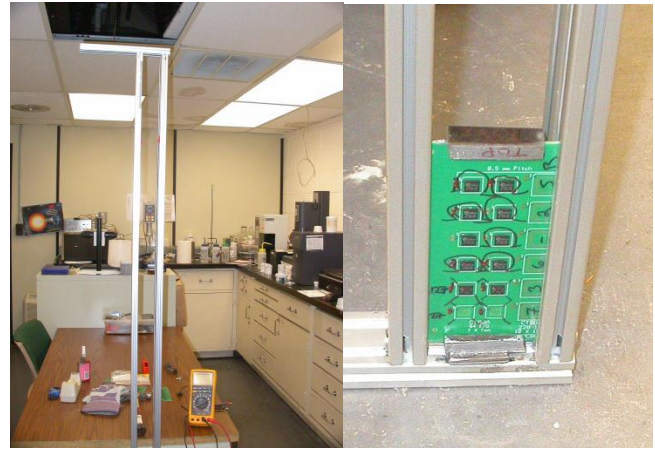
Figure 15 Frame for drop test setup (left), with a test board already landed on the bottom of test frame (right).
