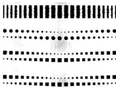
Figure 22 - Worst Stencil for Bottom Side Paste Smear
