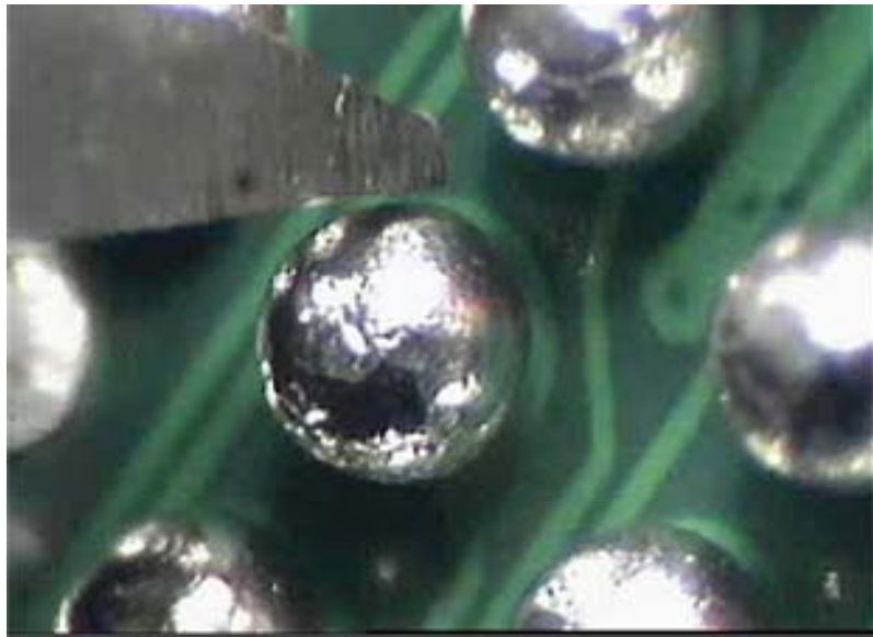
BGA Ball Shearing Test Four point bending test fixture and setup
