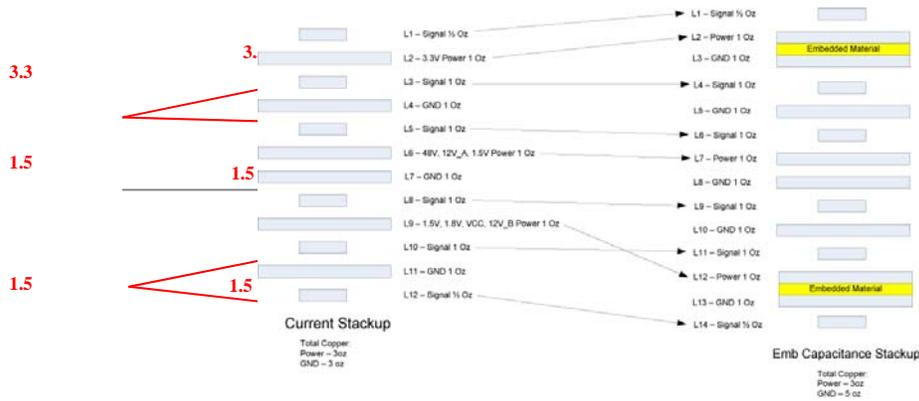
**Figure 1 - Adding embedded capacitance layers.**
