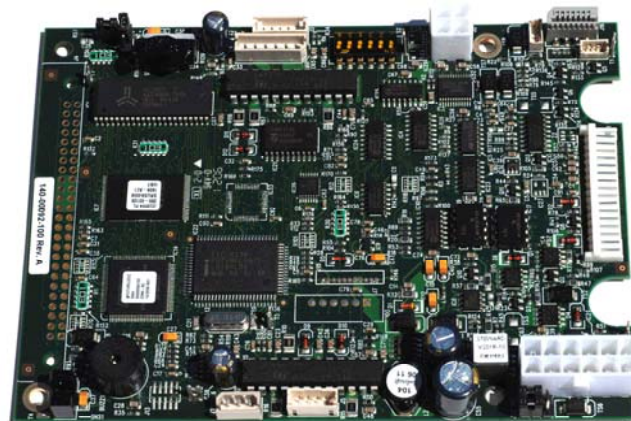
Figure 4 - K100 and SAC305 PCB
