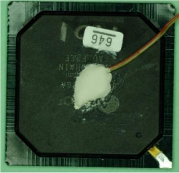
To characterize temperature on BGA parts, a hole was drilled into a sample part and a thermocouple was mounted just above the internal die.
