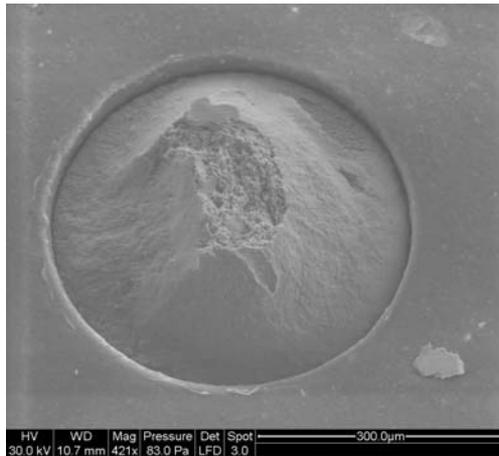
**Ball failure of Non-Reballed 676 I/O BGA**
