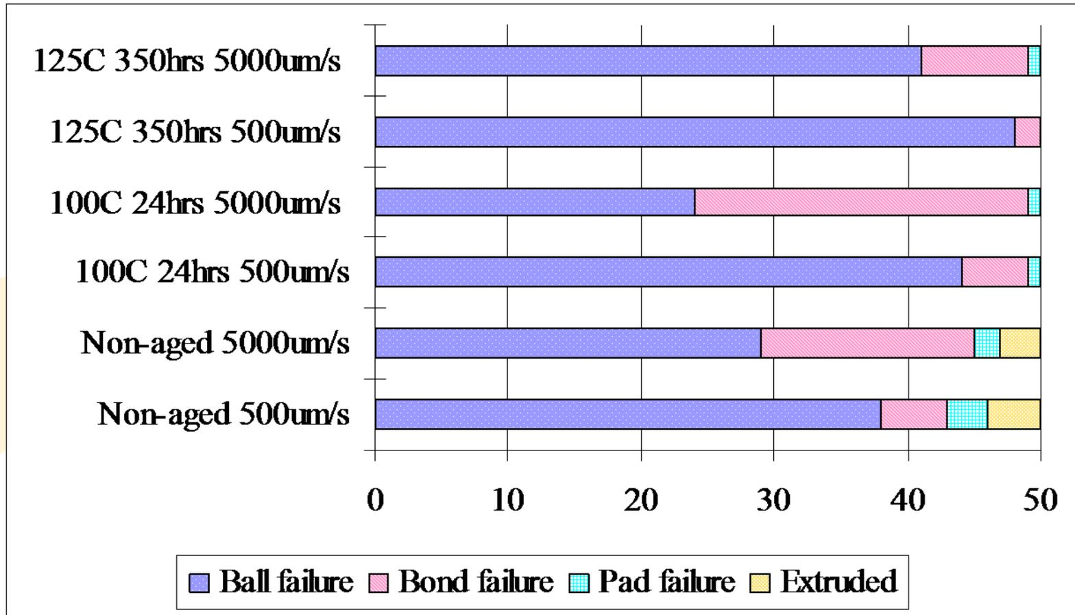
**The higher pull speed generated a greater number of bond failures.**
