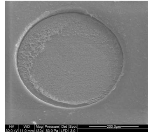
**Bond failure of Non-Reballed 676 I/O BGA**
