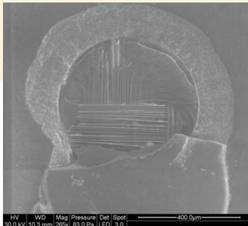
**Pad failure of Non-Reballed 676 I/O BGA**
