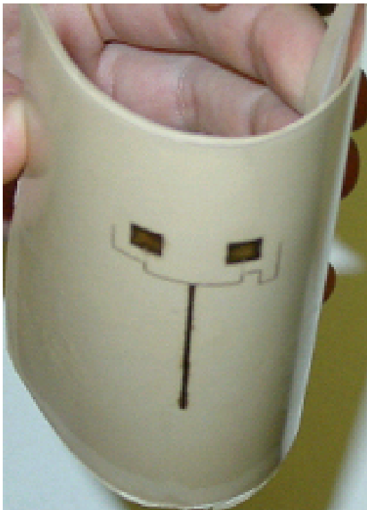
Flexible LCP circuit used as an antenna
