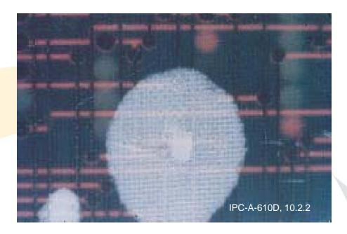
• Baking before soldering prevents damage
