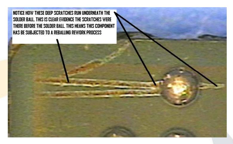
YOU SHOULD NEVER SEE SCRATCHES RUNNING UNDERNEATH BGA SPHERES OR TOP SURFACE MARKINGS
