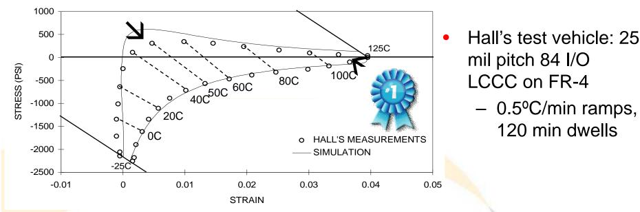
P. M. Hall's (AT&T) hysteresis loops gave SIGNIFICANT, QUANTITATIVE insight in the thermo-mechanical response of SnPb board assemblies
