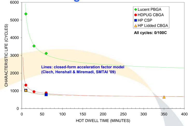
To figure out how fast saturation occurs, need thermal cycling failure data as a function of dwell time
