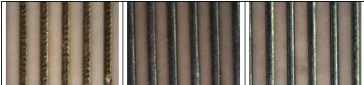
Soldered residues – not removed
