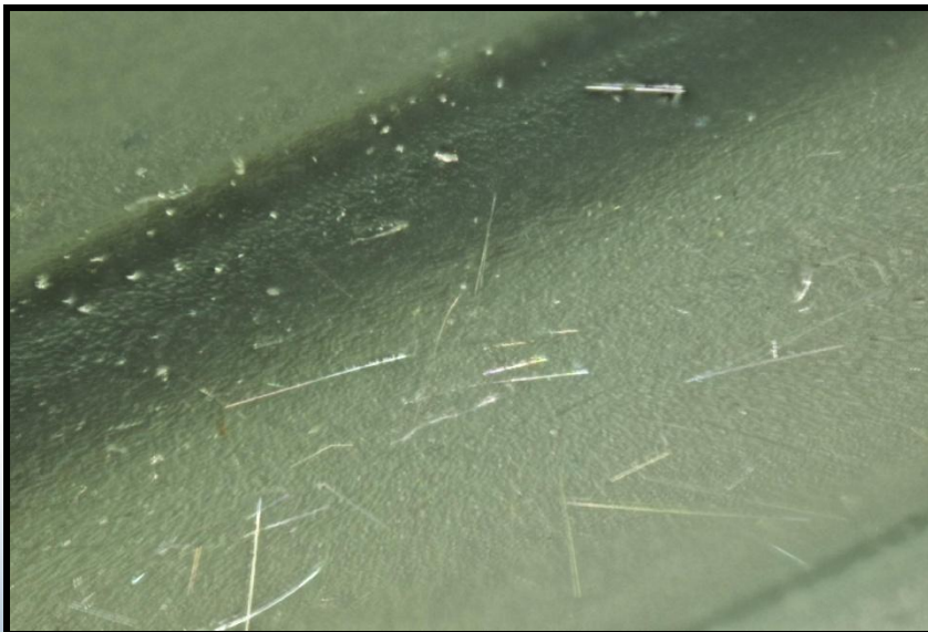
Entire surface of bracket is covered with tin whiskers
