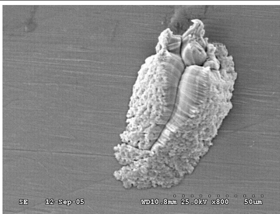
CU-A-1 06 Whisker forming from hillock surface
