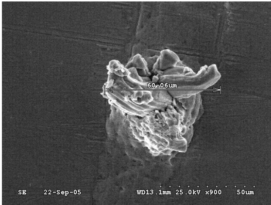
CU-U-2 06 Whisker forming from hillock surface - Protruding 60 um diameter hillock
