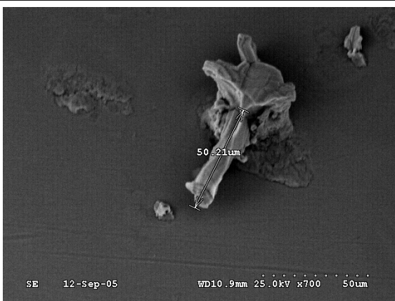
CU-A-1 06 Straight whisker formation from a hillock surface – Protruding 50.2 um
