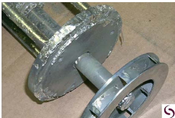
Figure 1 – Unprotected Stainless Steel
