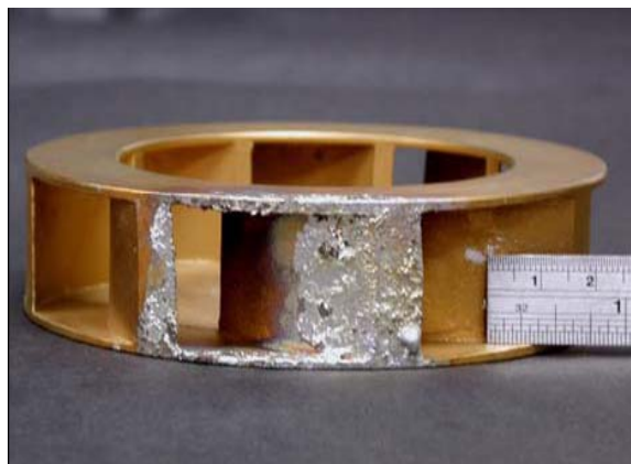
Figure 6 – TiN coated 316 stainless steel impellor
