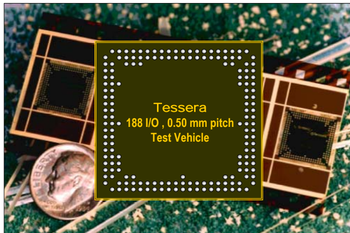
Circa 1994-Single metal layer, polyimide tape based substrate
