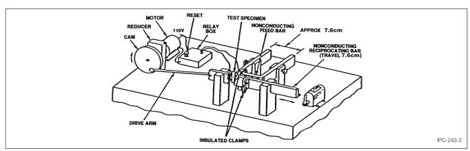
Figure 2 Typical Flexural Endurance Test Fixture Equipment
