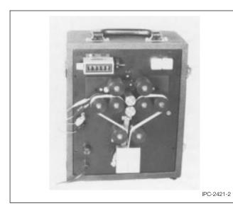
Figure 2 Fatigue ductility flex tester
