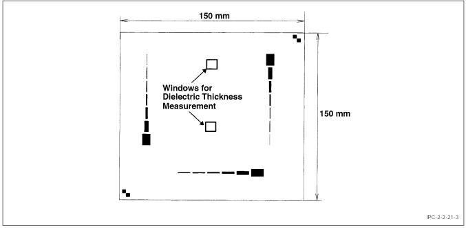
Figure 3 Pattern of One Test Board Showing Three Test Substructures (Board is 150 mm sq.)
