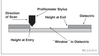
Figure 4 Cross Section of Window Used for Dielectric Thickness Measurement
