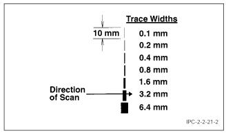
Figure 2 Top View of Planarization Structure
