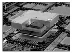
The DataStar Supercomputing cluster at the San Diego Supercomputer Center has 2464 processors and is the 35th most powerful supercomputer in the world. One DataStar node, the IBM p655+, employs an 8-processor Power4+ -based multichip module (shown above), that consists of four integrated dual-core chips. Source: University of California, San Diego, Dept. of Computer Science and Engineering (www-cse. ucsd.edu/).
