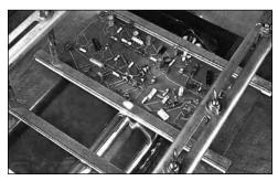
Early wave soldering of a through hole demo board, late 1960s
