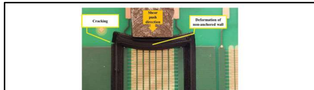
Figure 24. Deformation and Cracking of ABS Wall Structure during Shear due to Superior Mechanical Anchoring of Filled 0.8 mm Grooves. Specimen Printed using 0.8 mm Diameter Extrusion Nozzle.
