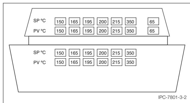
**Figure 3-2 Example of Reflow Oven Recipe Set Points**
