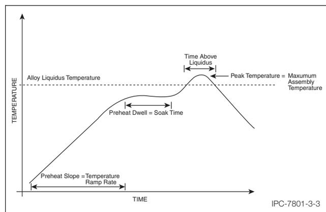
**Figure 3-3 Zones in a Typical Reflow Profile**
