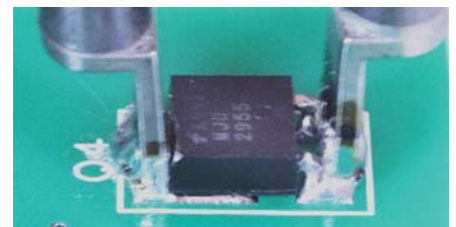
Figure 4 Confirm Solder Melt and Lift Component.
