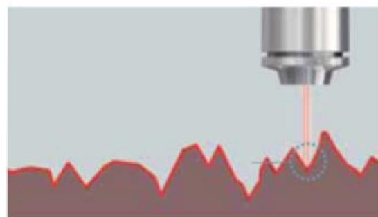
High mag lens, smaller beam spot, low S-filter value
