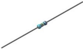
**Figure 8-1 Axial Resistor**
