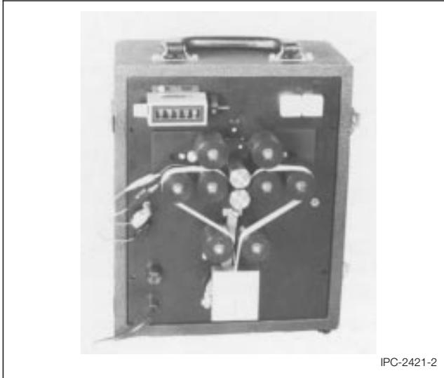
**Figure 2 Fatigue ductility flex tester**
