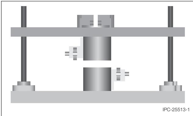
**Figure 1 Split-Cylinder Resonator**
