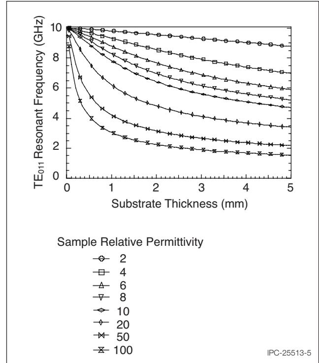
**Figure 5 Frequency of the  $TE_{011}$  Resonant Mode as a Function of Permittivity and Substrate Thickness for the 10 GHz Split-Cylinder Resonator**
