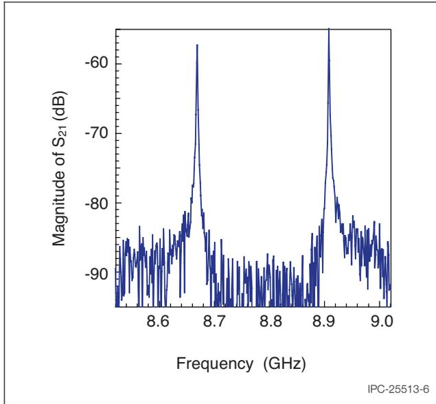
**Figure 6 Typical Multiple Split-Cylinder Resonator Resonances**
