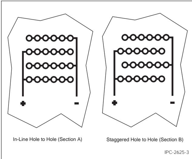
**Figure 3 CAF Test Board PTH-PTH Spacing Design**
