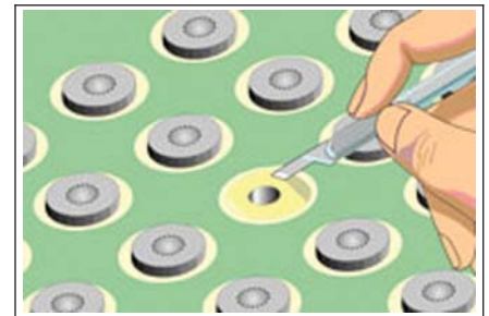
Figure 1 Remove the defective land and prepare connecting via.
