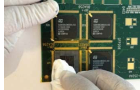
Figure 6 Wipe off excess solder paste
