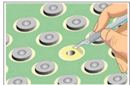
Figure 2 Remove the defective land and prepare connecting via.
